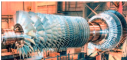
Nonlinear thermomechanical calculation of a combustion turbine compressor: bladed rotor and quarter compressor.
